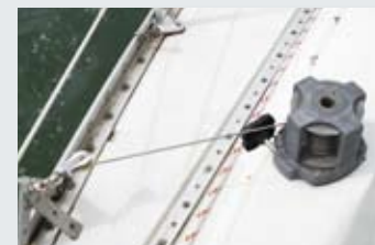
Clockwise from top left: The wire furling line and dedicated winch works well, but watch your fingers; the heads is very roomy for an older boat with plenty of storage and room to move about in; having the primary winches and mainsheet traveller all to hand from the helm means singlehanded is simple.
